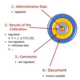
Figure 2: DCC structure [1]
